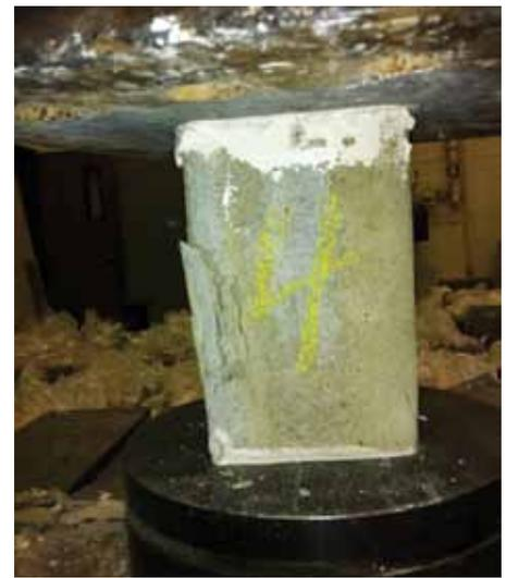
Figure 3: Grout samples during testing.
