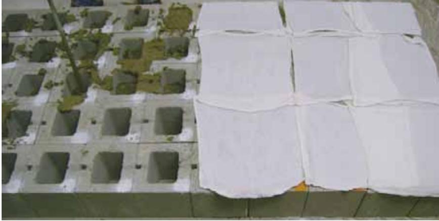
Figure 2: Grout samples during casting.
